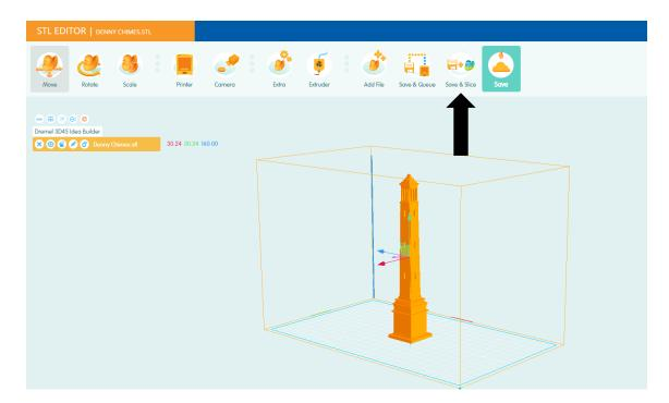
6. In the next window, the Dremel 3D45 Idea Builder should be selected under the printer type. Under slicing profile, select "PLA with cost estimate". Set your layer thickness, shell thickness, and infill for your part. Uncheck "supports" if you do not think the part needs them. Then click "slice".
